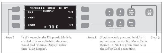
FIGURE 33: Enabling/Disabling the Diagnostic Mode
